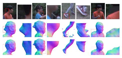
Fig. 7. Our approach improves the 3D reconstruction accuracy. First row: reference input image. Second row: reconstructed 3D model using the 3D point cloud from PMVS [12]. Third row: reconstructed 3D model using our refined 3D point locations of the 3D point cloud.
