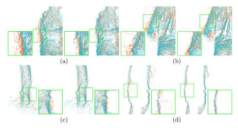
**Fig. 8.** We translate the point cloud at t (orange points) to match with the point cloud at t + 1 (cyan points) according to the estimated scene flow. We show the zoom-in regions for: (a) man's back (b) arm part (c) ankle part. (d) Vertical cross section of human's torso. As we can see from the figure, the orange points align well with the cyan points which shows that our estimated scene flow is accurate.
